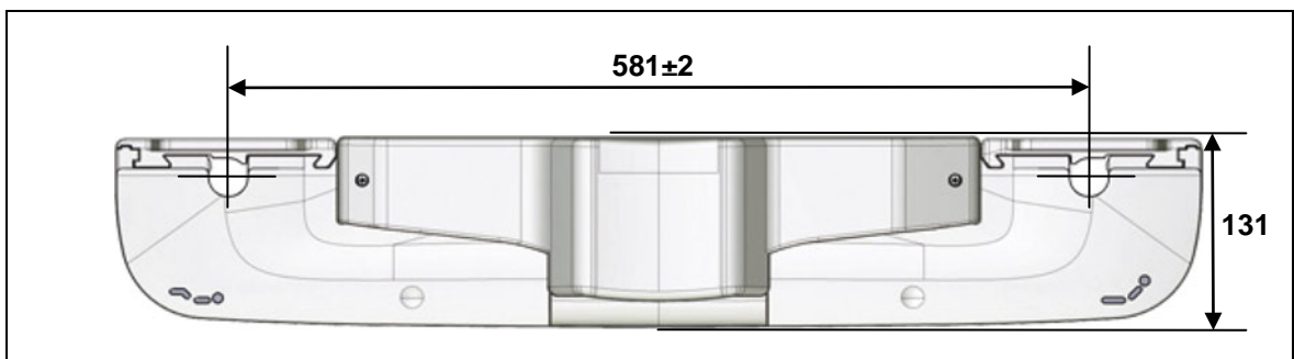
Figure 10 Dimensions of the DUOMAT 9 drive, in mm
