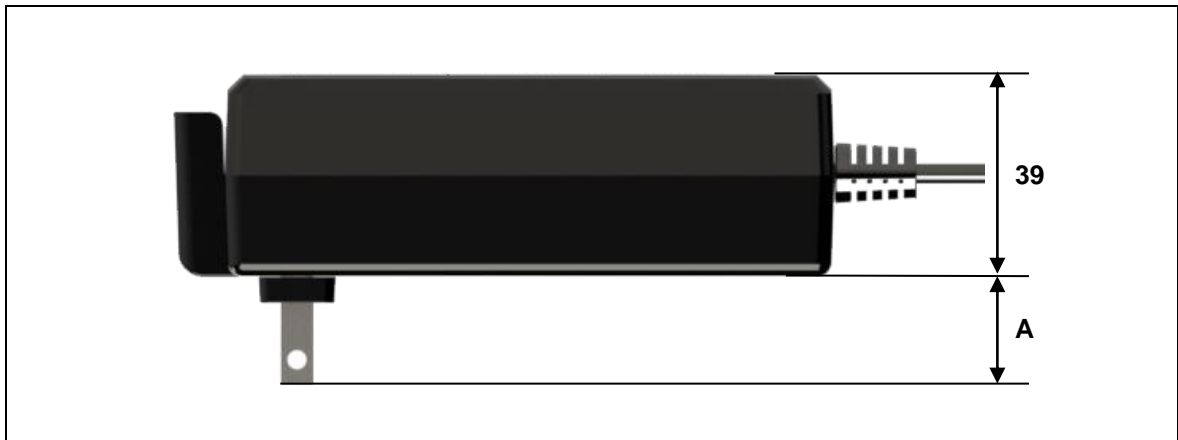
Figure 7 Dimensions of the PD23, side view (in mm)
