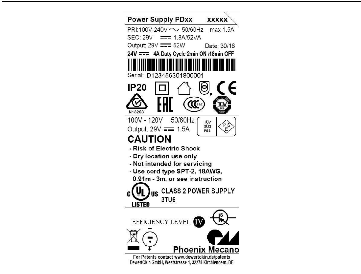
Figure 2 Example: Ratings plate for the PD12/PD13 POWER SUPPLY
