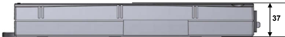
Figure 43 COMPACT control unit, side view (in mm)
