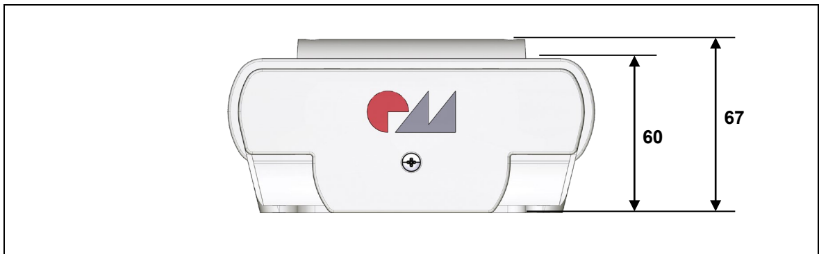
Figure 7 Dimensions of the ECS control unit, front view (in mm)
